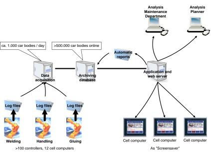
In the current state of development, the database is protected against malfunctions by replication, making it a highly available computer system.
